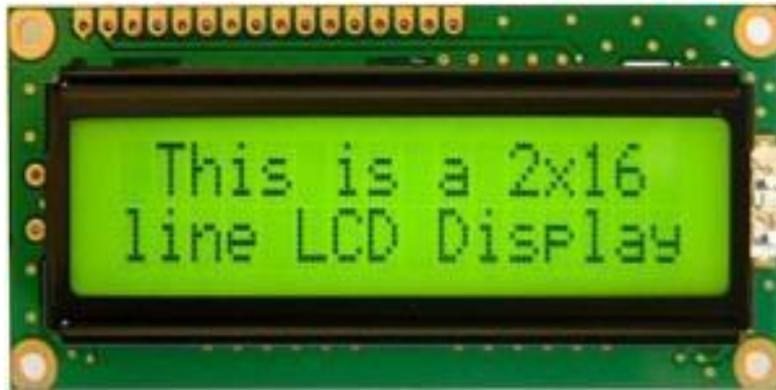
**Gambar 1.** Modul LCD 2x16
